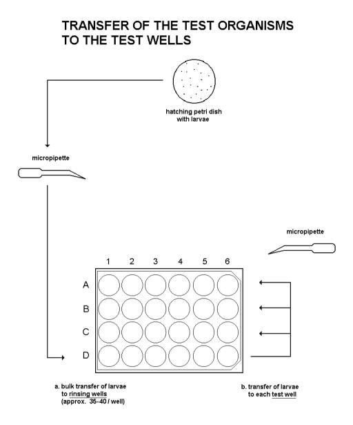
The next steps are executed under a dissection microscope at magnification 10-12x, or alternatively on a light box with a magnifying glass (6-8 x).
