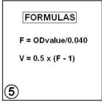
calculate dilution factor F and dilution volume V
