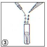
transfer ciliate suspension into stock-culture cell and add 1 ml distilled water
