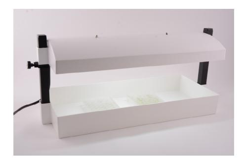
Table top Light Unit for incorparation in an incubator or temperature controlled room at 25 °C. Uniform illumination with full spectrum grow lights for optimal growth of the duckweed.
