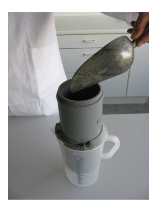
Fill the sediment press to half of its contents with sediment or sludge
