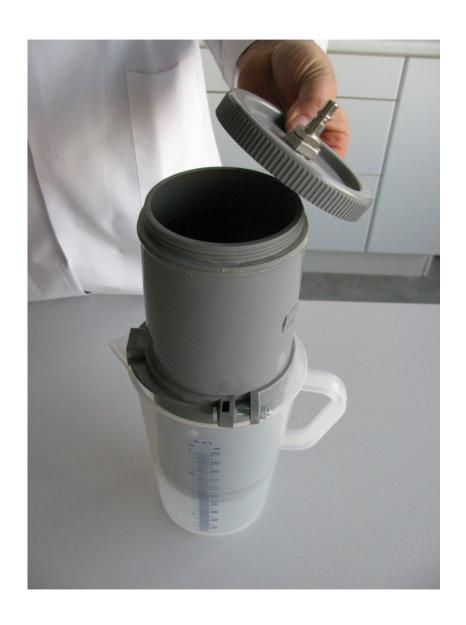
Put the lid back on top of the sediment press
