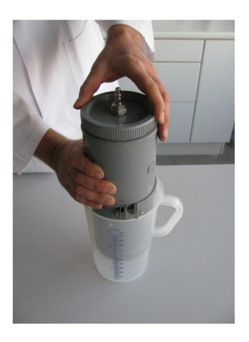
Screw the lid firmly on the cylinder to close the sediment press tightly
