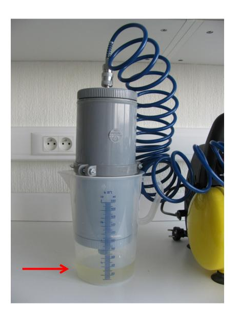
The pore water will slowly drop from the tube at the bottom of the cylinder, into the collecting container
