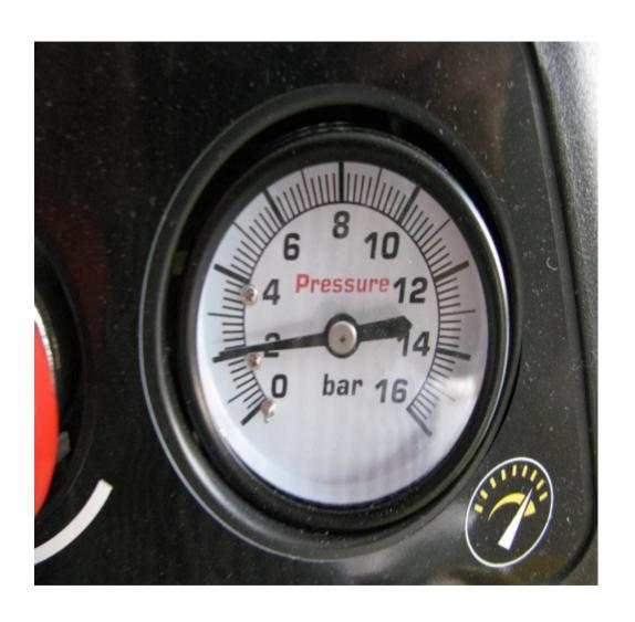
Adjust the pressure of the compressor to a maximum of 2 bar
