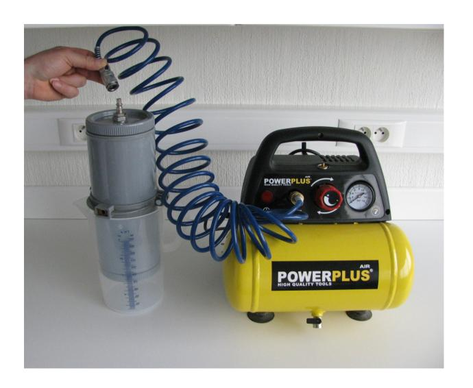
Connect the sediment press to the air compressor
