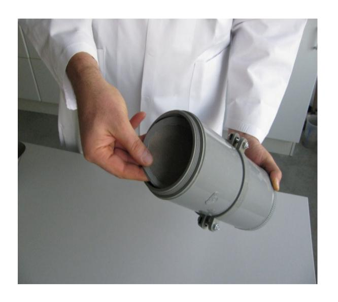
Put the stainless steel grid filter disc in the sediment press and push it down to the bottom of the cylinder
