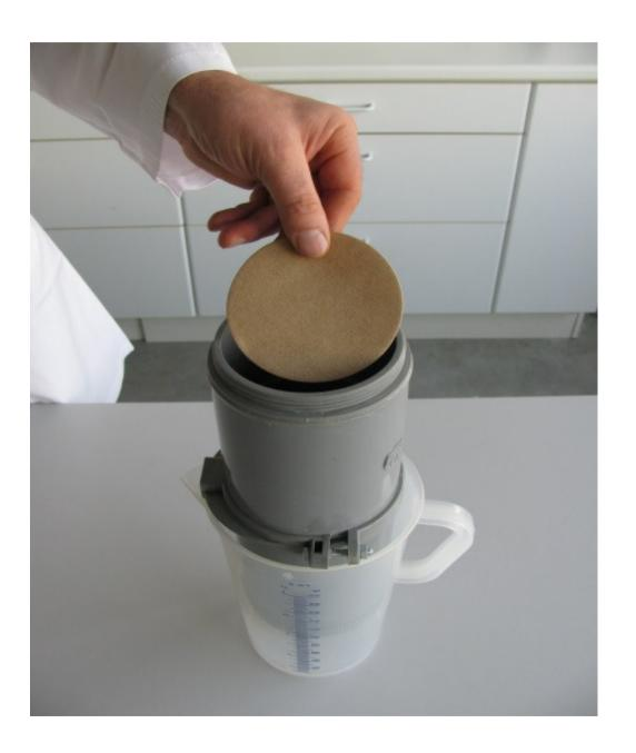
Put the filter paper disc in the sediment press and push it down to the bottom, onto the stainless steel grid filter disc.
