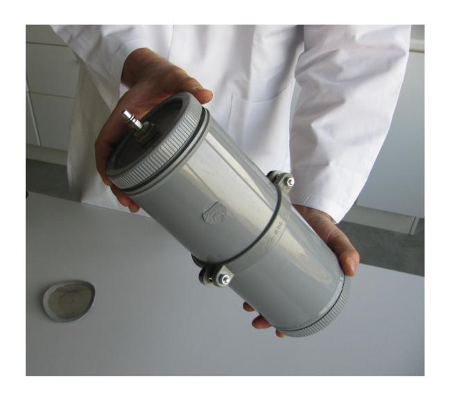
Screw off the lid at the top of the sediment press
