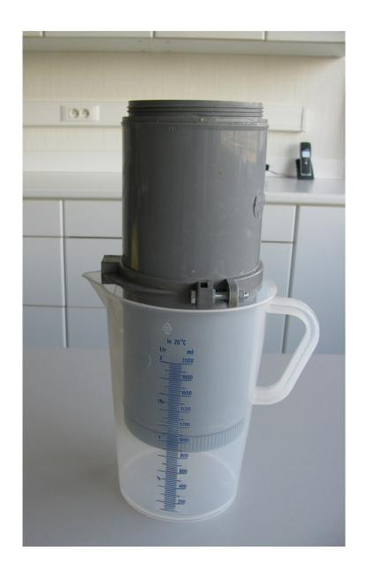
Put the sediment press vertically in the pore water collecting container untill the ring in the middle of the press rests on the edge of the container
