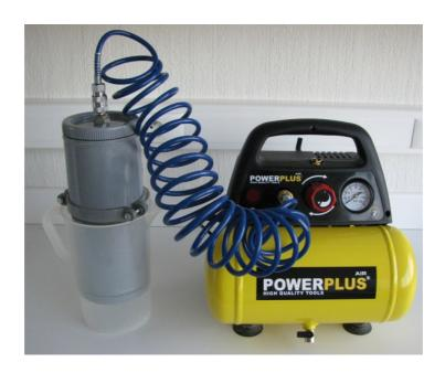
The sediment press consists of a cylinder in PVC, closed at the top with a removable lid provided with a connection for coupling of the press to an air compressor.
