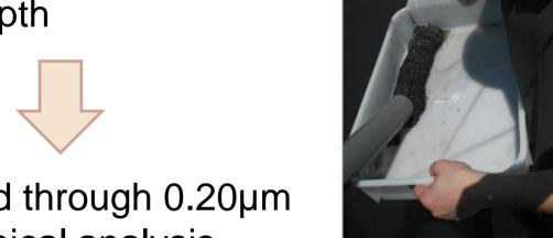
Filtered through 0.20µm for chemical analysis
