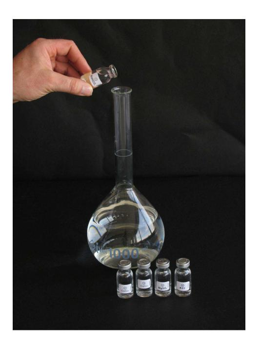
POUR THE 5 VIALS WITH CONCENTRATED SALT SOLUTIONS IN  $\pm$  800 ML DISTILLED WATER, IN THE 1 LITER VOLUMETRIC FLASK
