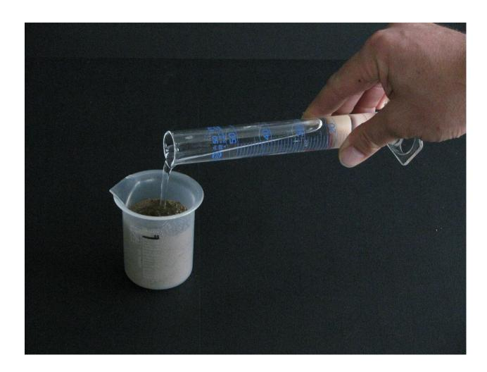
POUR THE  $\underline{\bf 50}$  ml water in the beaker with the soil
