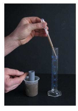
SUCK UP THE SUPERNATANT FROM THE MICROSIEVE WITH THE WIDE MOUTH MICROPIPETTE AND TRANSFER IT INTO THE GRADUATED CYLINDER
