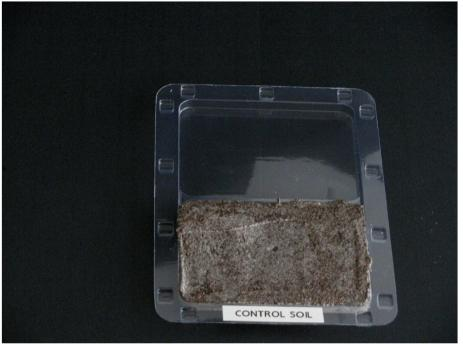
FLATTEN THE SURFACE OF THE SOIL TO OBTAIN A LAYER OF UNIFORM DEPTH
